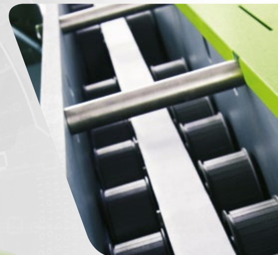
Roller drive with 2 servomotors
