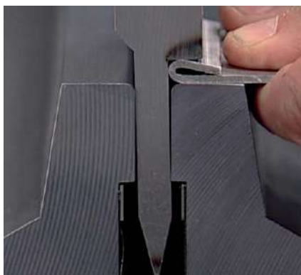
Pre-bend and flattening in the same tool.
