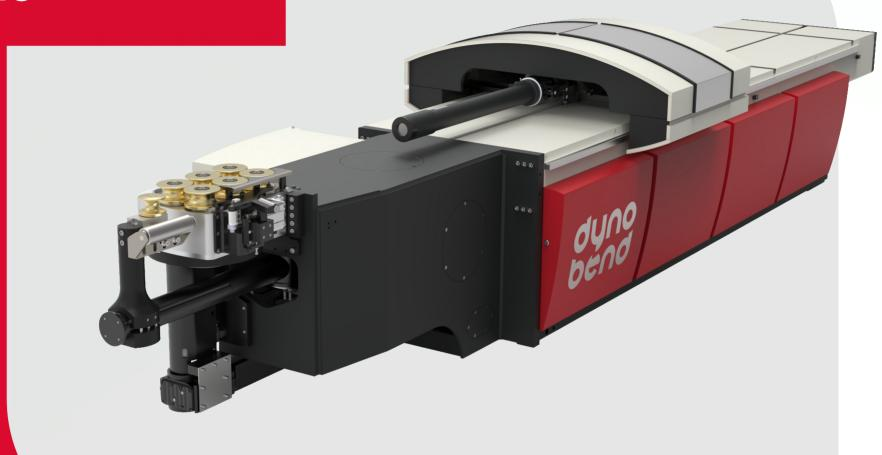
Free Form bending machine (V)
